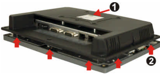
Figure 1-2: SP-xx00-72 Plastic Back Cover Removal
